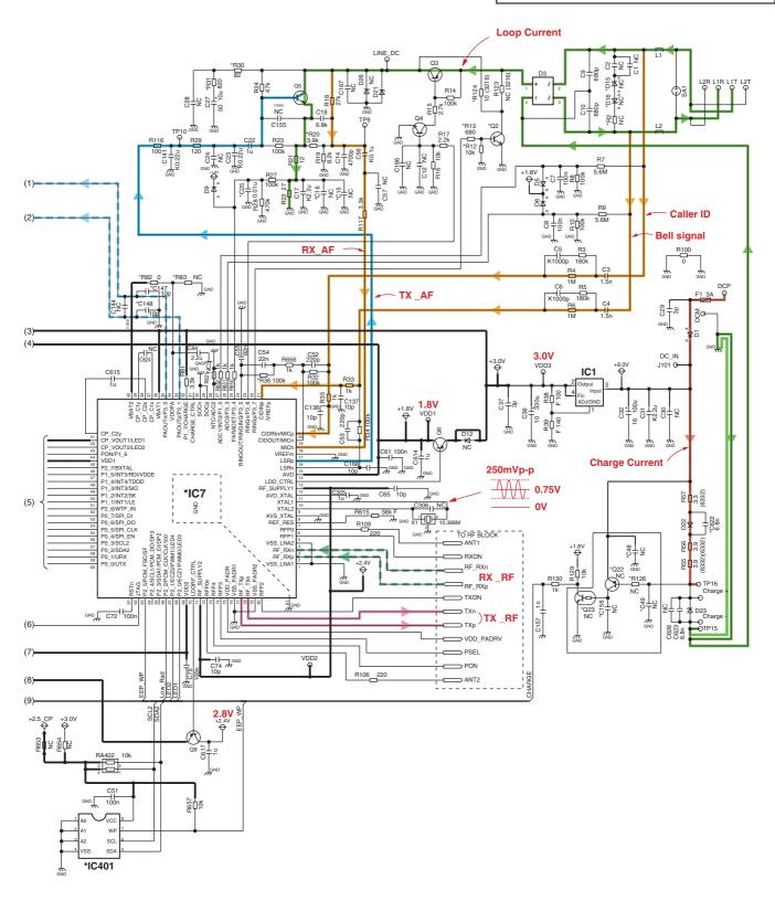
NC: No Components KX-TG8021BX SCHEMATIC DIAGRAM (Base Unit)
