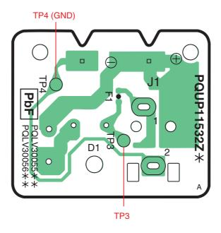
CIRCUIT BOARD (Charger unit (Bottom View))
