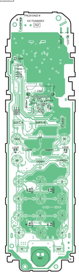
KX-TGA800 CIRCUIT BOARD (Handset\_Main (Bottom View))
