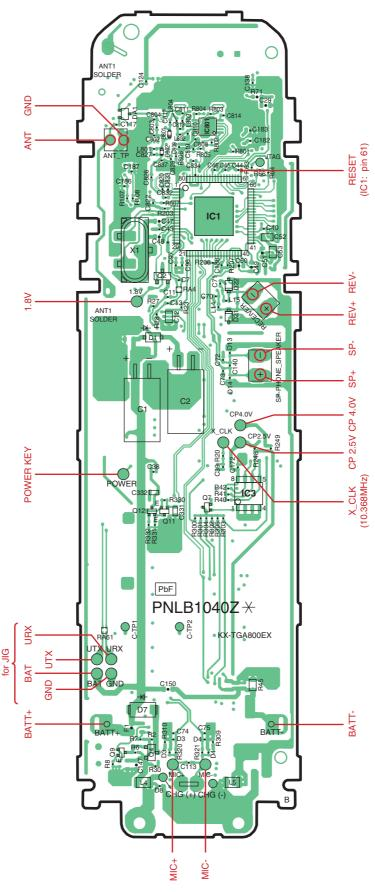
KX-TGA800 CIRCUIT BOARD (Handset\_Main (Component View))
