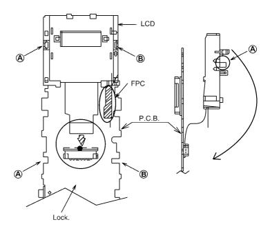
2 Locate the Flat Cable inside as shown.
