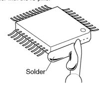
When you attach a new IC to the board, remove all solder left on the board with some tools like a soldering wire. If some solder is left at the joint on the board, the new IC will not be attached properly.
