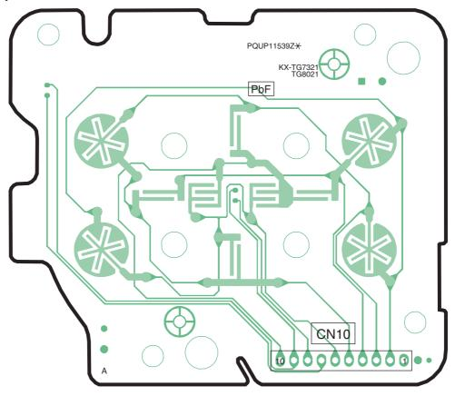
KX-TG8021 CIRCUIT BOARD (Base Unit\_Operation (Component View))
