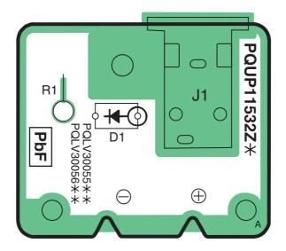
CIRCUIT BOARD (Charger unit (Component View))
