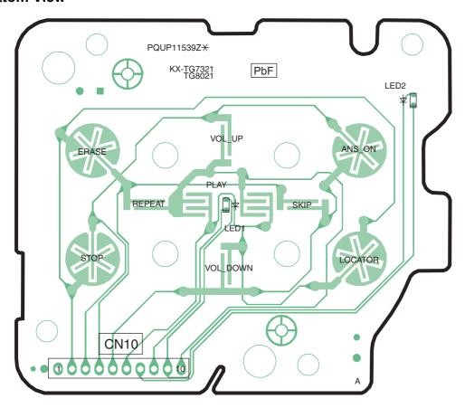
KX-TG8021 CIRCUIT BOARD (Base Unit\_Operation (Bottom View))
