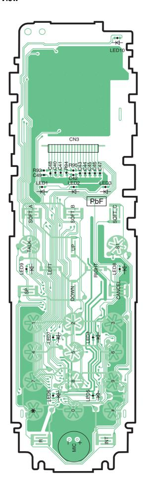
KX-TGA710 CIRCUIT BOARD (Handset (Flow Solder Side View))
