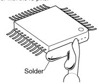
When you attach a new IC to the board, remove all solder left on the land with some tools like a soldering wire. If some solder is left at the joint on the board, the new IC will not be attached properly.
