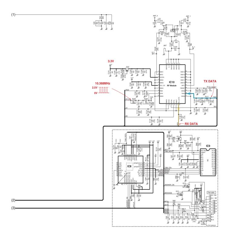
NC: No Components KX-TG7100BX SCHEMATIC DIAGRAM (Base Unit)
