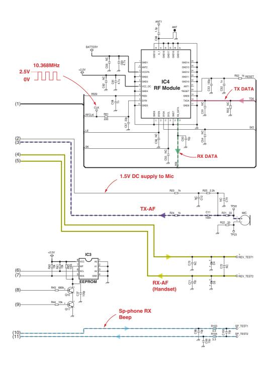
NC: No Components KX-TGA710 SCHEMATIC DIAGRAM (Handset) KX-TG7100BXS/KX-TG7100BXT/KX-TGA710CXS/KX-TGA710CXT
