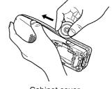
4 Remove the cabinet cover by pushing it upward.
