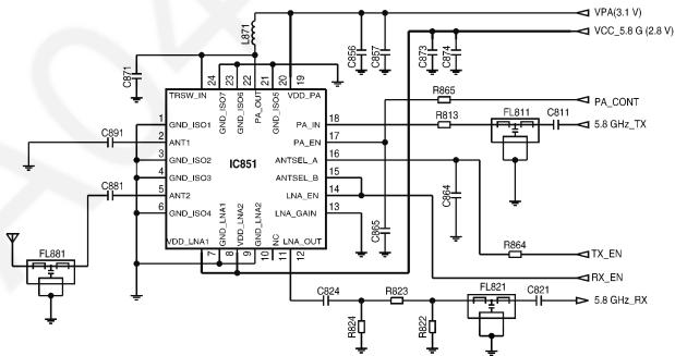
IC851 includes Switch for High frequency signals, and controlled by PA\_CONT signal and RX\_EN signal from DSP. At the TX mode 5.8 GHz TX signal from 5.8 GHz PA block leads to Antenna terminal, at the RX mode 5.8 GHz RX signal from Antenna terminal leads to 5.8 GHz LNA block.
