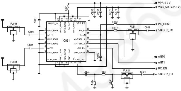
IC851 includes Switches for High frequency signals, and controlled by ANT0 signal and ANT1 signal from DSP. DSP is checking RSSI (Received Signal Strength Indicator) signal, and selects better condition Antenna from two antennas. At the TX mode 5.8 GHz TX signal from 5.8 GHz PA block leads to selected Antenna terminal, at the RX mode 5.8 GHz RX signal from selected Antenna terminal leads to 5.8 GHz LNA block.
