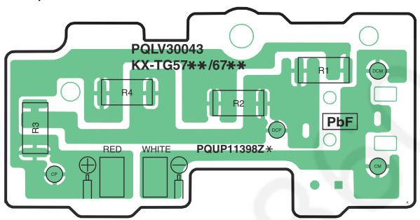
CIRCUIT BOARD (Charger Unit (Component View))
