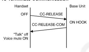
When the OFF button on the Handset is pressed during communication, a LINK terminating DATA (CC-RELEASE) is sent to terminate the communication. Then DATA (CC-RELEASE-COM) is returned from Base Unit. Handset receives it and reset the link.
