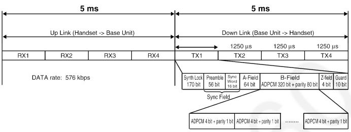
Sync Field (72 bit): Preamble 56 bit + SyncWord 16 bit
