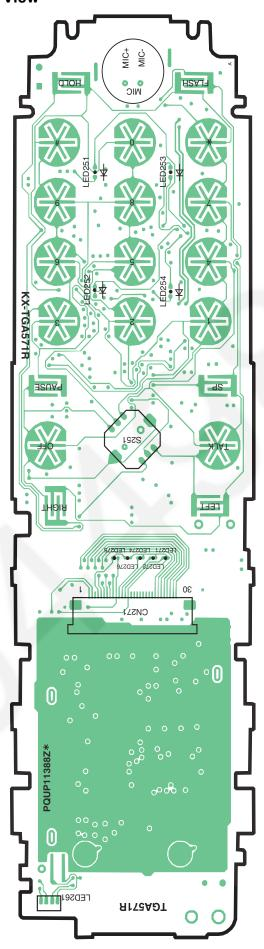
KX-TGA571 CIRCUIT BOARD (Handset\_Main (Flow Solder Side View))
