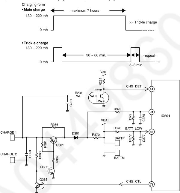
Pin 87 of IC201 monitors the battery voltage and detect BATT LOW at 2.34 V.
