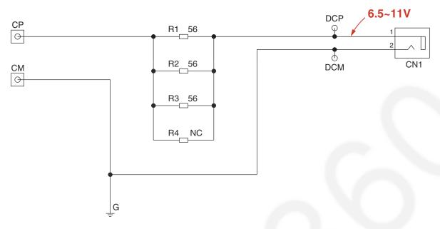
NC: No Components SCHEMATIC DIAGRAM (Charger Unit)
