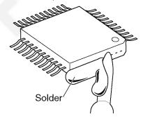
When you attach a new IC to the board, remove all solder left on the land with some tools like a soldering wire. If some solder is left at the joint on the board, the new IC will not be attached properly.
