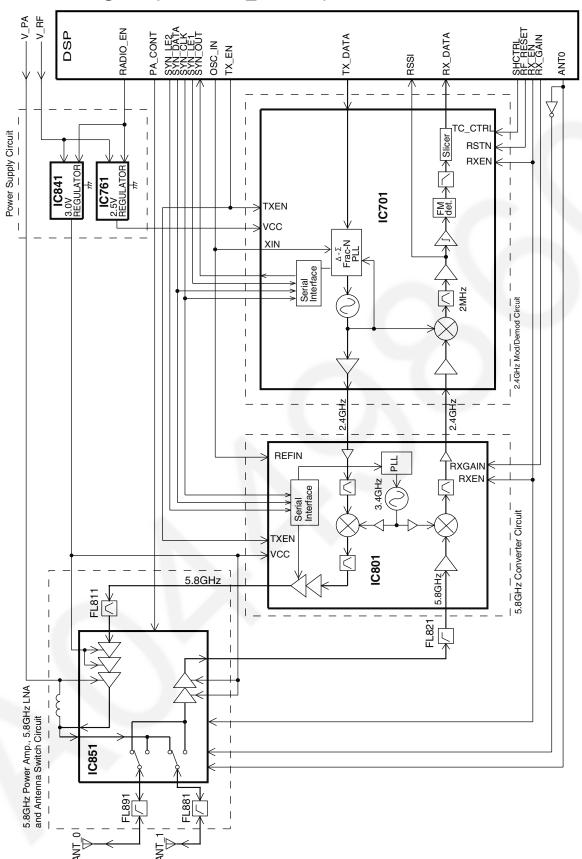
KX-TG5776/5777 BLOCK DIAGRAM (Base Unit\_RF Part)
