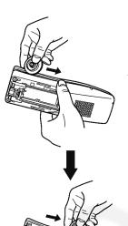
Insert a JIG (PQDJ10006Y) between the Cabinet Body and the Cabinet Cover, then pull it along the gap to open the Cabinet.
