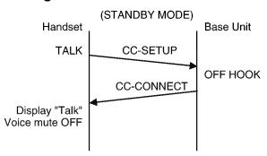
When calling, a communication request DATA (CC-SETUP) is transmitted from the Handset, and a permitting DATA (CC-CONNECT) is returned from the Base Unit to it. At that time the audio path opens.
