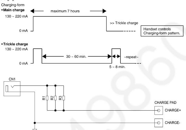
The route for this is as follows: DC+pin of CN1 $\rightarrow$ R1  $\sim$  R3 $\rightarrow$ CHARGE+pad $\rightarrow$ Handset $\rightarrow$ CHARGE-pad $\rightarrow$ DC-pin of CN1.
