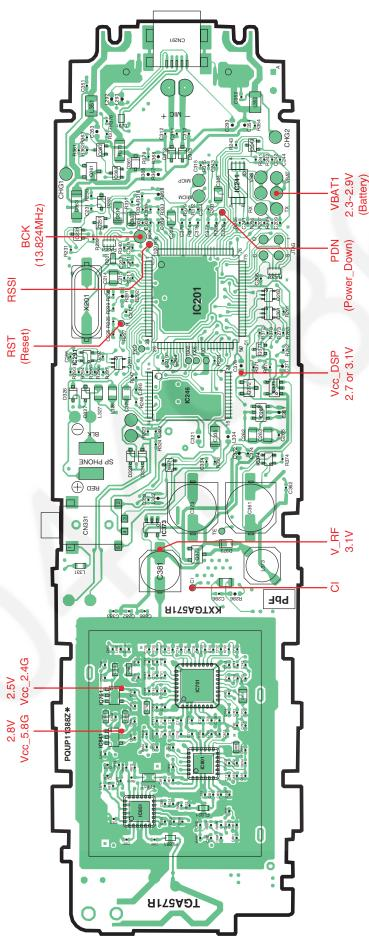
KX-TGA571 CIRCUIT BOARD (Handset\_Main (Component View))
