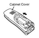
Remove the Cabinet Cover by pushing it upward.
