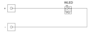
KX-TG3821/3822 SCHEMATIC DIAGRAM (Base Unit\_LED)
