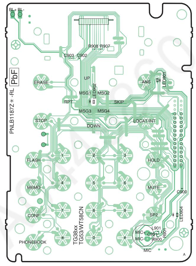
KX-TG3821 CIRCUIT BOARD (Base Unit\_Operation (Component View))
