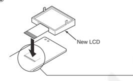
Fit the heatseal of a new LCD.
