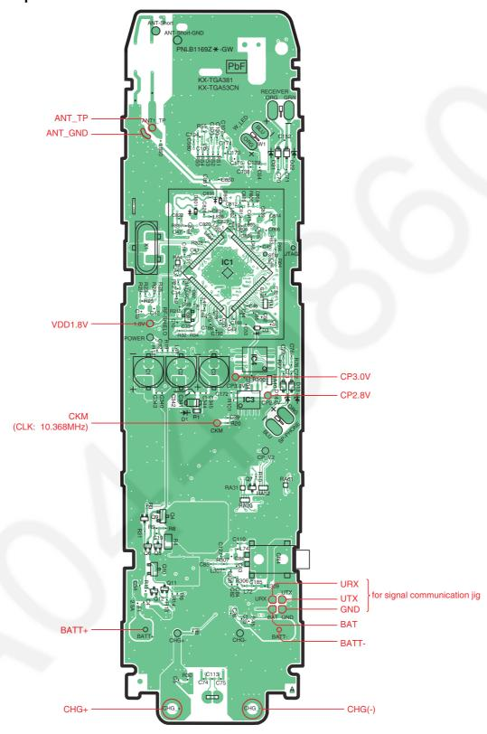
KX-TGA381 CIRCUIT BOARD (Handset\_Main (Component View))
