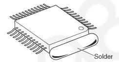
2. Make a few cuts into the joint (between the IC and its pins) first and then cut off the pins thoroughly.
