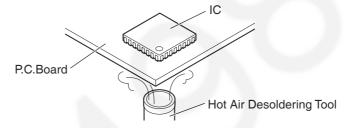
2. Pick up the IC with tweezers, etc. when the solder is melted completely.
