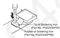
Heatweld with the tip of the soldering iron about 5 to 8 seconds (in case of 60W soldering iron).
