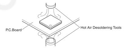
3. After removing the IC, clean the P.C.Board of residual solder.
