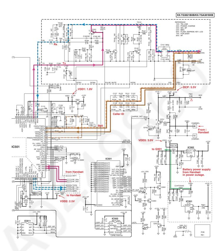
NC: No Components KX-TG3821BX SCHEMATIC DIAGRAM (Base Unit\_Main)
