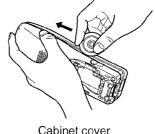
Remove the cabinet cover by pushing it upward.
