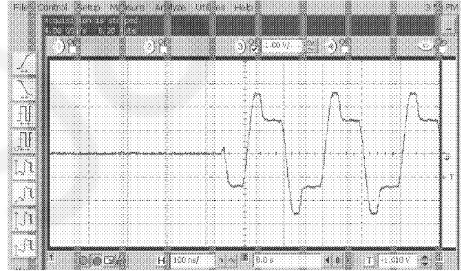
3-④ 10Base-T waveform 4 [ during data communication ] (A part of the waveform 3 is magnified.)
