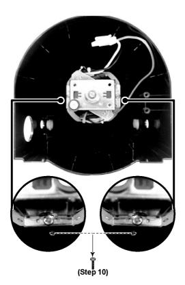
Step 11 Remove Connector Complete.
