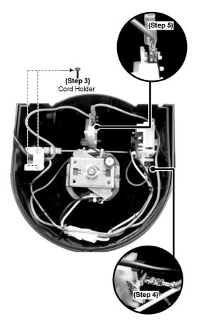
Step 6 Detach Connector.Step 7 Remove Switch Assy.
