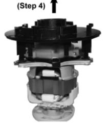
Step 5 Remove 3 Screws and pull up the part.
