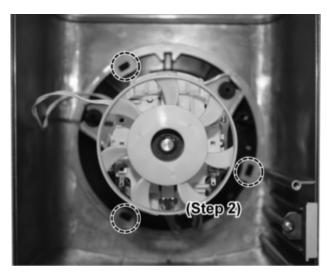
Step 3 Hold the bottom side and turn the Top Side toclockwise and release the Motor Unit.
