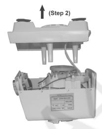
Step 3 Remove 3 Screws. Step 4 Take out the Dressing Box Cover.
