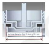
Seal outer diameter: From 52.6mm to 53.2mm
