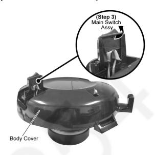
Step 4 Release Wires from Wire Holder.
