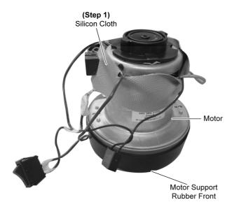
Step 2 Release Wire Connectors from Motor.
