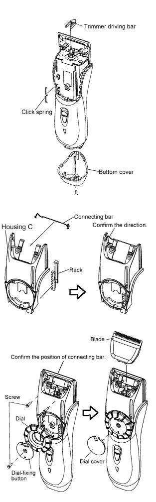
10. Attach the connecting bar to housing C.
