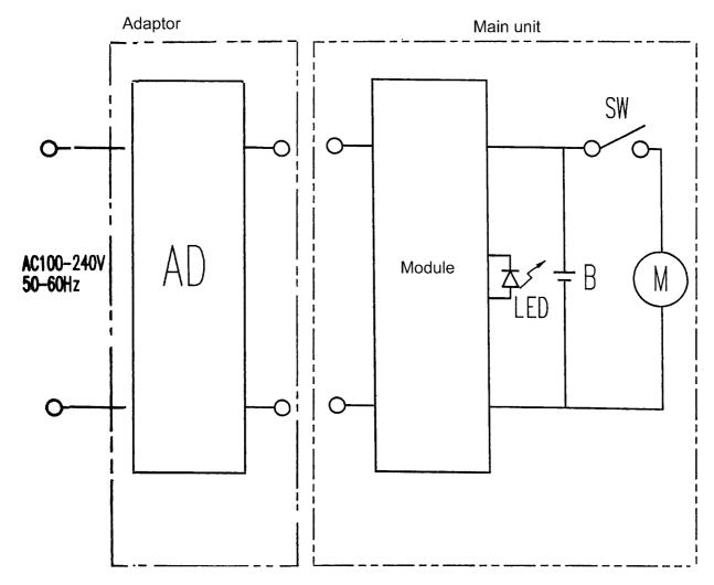
**2 WIRING CONNECTION DIAGRAM**
