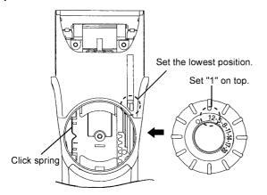
After assembling the unit, confirm the smooth up and down operation for attachment. And confirm if the dial shows "20" when the attachment is the highest position.
