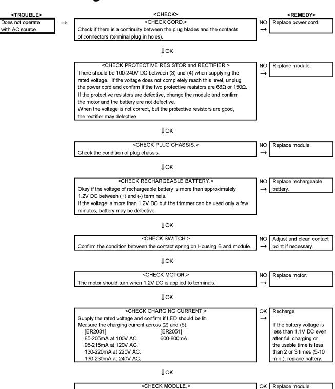
It is OI if the motor rotates and LED is lit when the switch is ON.
