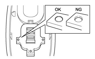
3. Insert the terminal pins into the hole of housing A firmly and set the battery & module assembly into the housing A.
