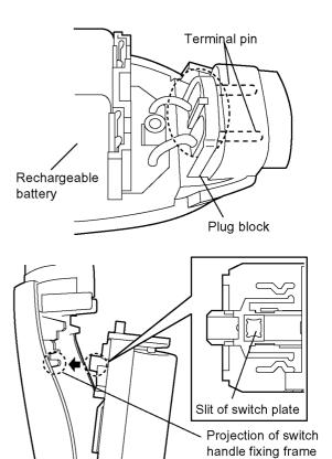
4. Insert the motor facing the sticker on the housing B side.
