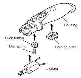
2. Place the holding plate on the housing A firmly.
