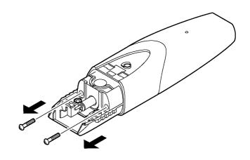
8. Remove the housing A. **NOTE:** Make sure not to lose two screw O-rings.
