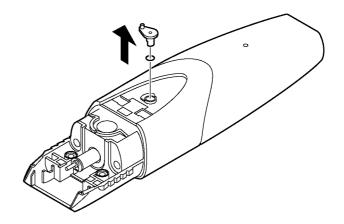
5. Take out the switch cam and the O-ring. **NOTE:**
