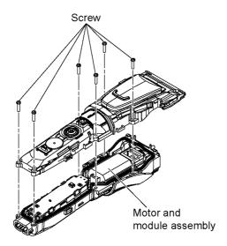
10. Pull the chassis and module assembly upward.
