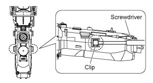
9. Loosen 6 screws and remove the motor and module assembly.
