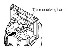
4. Loosen a screw on bottom and slide down the bottom cover.
