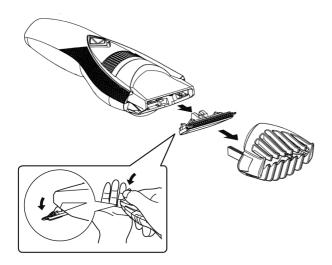
2. Loosen two screws and remove the blade holder.
