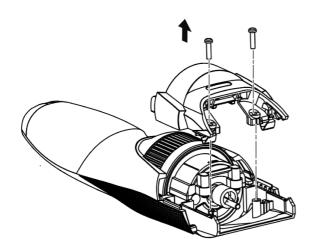
3. Loosen a screw from bottom cover.
