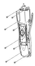
7. Separate the housing B from the housing A.
