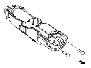
9. Remove the battery from the chassis.
