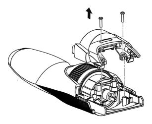
3. Loosen a screw from bottom cover.
