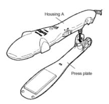
6. Remove 6 torque screws fastened the housing B from the housing A as shown in Figure 6.
