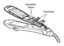
3. Remove the pivot shaft cover by using a straight-edge screw driver as shown in Figure 3.
