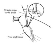
4. Remove a torque screw and the pivot shaft from housing as shown in Figure 4.
