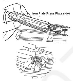
(9) Remove Slide Plate and Slide Spring.
