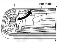
2 Take off Circuit by push at Hook of Housing B
