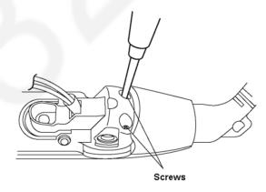
(12) Remove 6 Screws by Phllips screw driver (Plus Driver).
