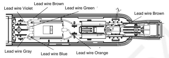
2. Arrange Lead wire into rib of Hosing A as shown in Figure
