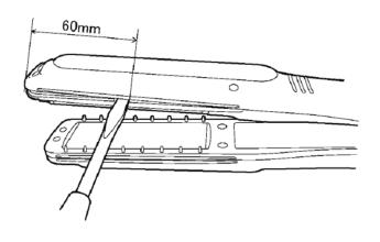
(7) Take off Iron Plate from Hook of Press Plate by slide.
