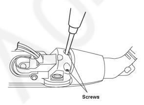
(10) Remove 6 Screws by Phllips screw driver (Plus Driver).
