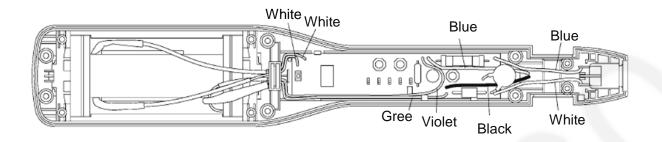
(2) Lead wire of Iron Plate(Heater B assembly b/k) arrangement follow as below.
