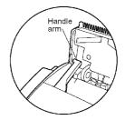
5. Set the linear motor assembly on the housing A and sliding it upward to hook. Confirm that the lead wire tube fits to the housing A firmly and no foreign substance sticking around. Attach the head block to housing A with care of the direction. And attach the rock lever shaft to housing B.
