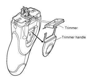
4. To remove the trimmer driving bar or the slit blade driving bar, press bars outward.
