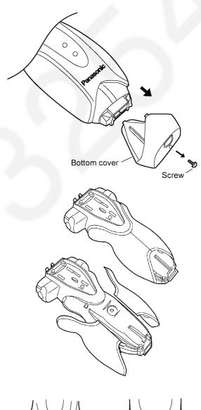
7. Loosen two screws on front and four screws on the back side, and remove two housing clips.
