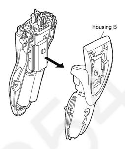
9. Remove the motor assembly and tube holder.
