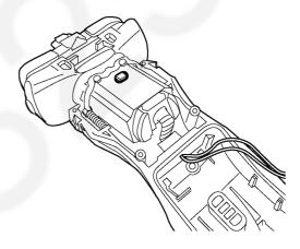
10. And take out the battery assembly from housing A.
