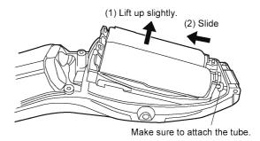
11. Remove the battery o-ring and washer in each battery. Take out the rechargeable batteries from the chassis.
