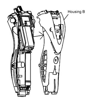
10. Remove the motor assembly first. And take out the module assembly from housing A.
