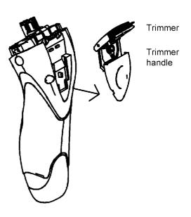
4. To remove the trimmer driving bar, press it outward.
