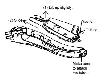
11. Remove the battery o-ring and washer from battery terminal. Take out the rechargeable battery from the chassis.
