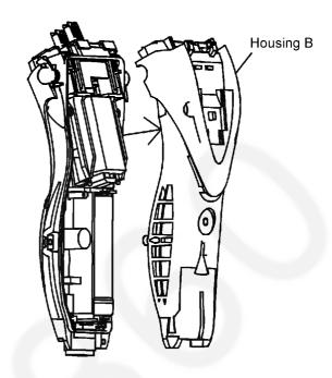
10. Remove the motor assembly first. And take out the module assembly from housing A.
