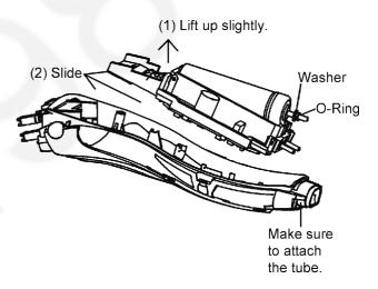
11. Remove the battery o-ring and washer from battery terminal. Take out the rechargeable battery from the chassis.
