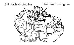
7. Remove the module and chassis assembly from the housing A.
