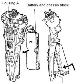
Insert the rechargeable battery into chassis. Confirm the direction of battery. Once battery is disassembled, the battery is reset. Connect the battery with the charging adaptor about 10 seconds first.
