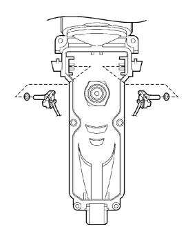
4. Before assembling the linear motor assembly to the housing A, attach the cleaning shutter from the bottom side.
