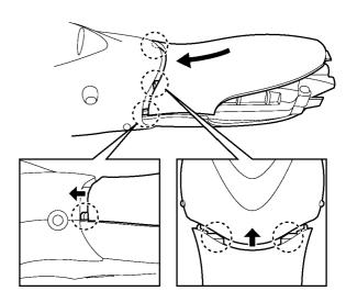
14. Tighten a screw with the bottom cover.
