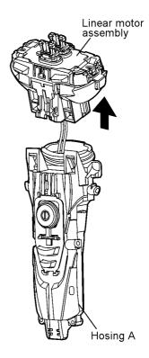
11. Unsolder the lead wires.
