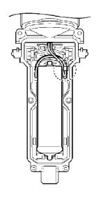
9. Set the trimmer driving bar and the slit blade driving bar.
