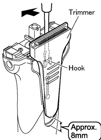
3. Remove the trimmer driving bar by pressing it outward.
