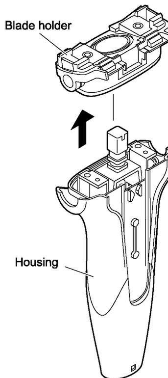
6. Set the switch to "OFF", and remove the chassis assembly from the housing.
