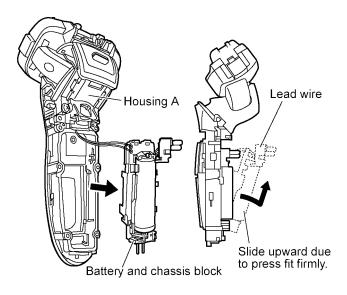
4. Make sure that the lead wires set in position to avoid abnormal noise. Install (+) terminal of battery into the terminal plate at the bottom cover side and firmly set the battery sliding the direction of arrow. Attach (-) terminal of battery.
