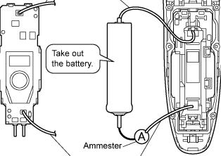
Lead wire of (+) side for checking charging current
