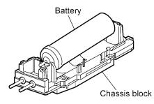
6. Unsolder the lead wires from the module.
