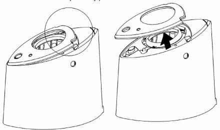
9. Unscrew three screws and remove the Ring and the Test switch rubber.
