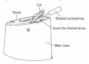
8. Close the Supply water lid and remove the Panel as the Figure. (Be careful to remove the both-side tape neatly.)
