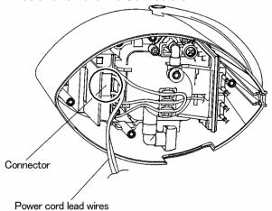
3. Remove the Blue lead wires
