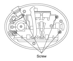
5. Loosen two screws and remove the boiler block.
