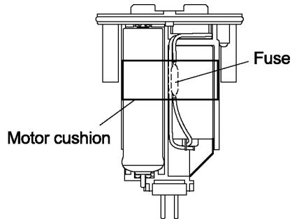
2. Press fit the lead wires into housing neatly.
