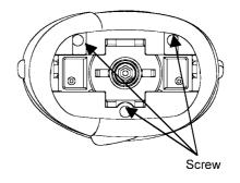
2. Remove the head mounting base, side panel, switch and switch cam. Remove the chassis with pushing the head release buttons.
