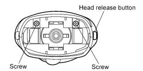
2. Take out the bottom cover with pushing a head release button.
