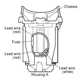
4. Close the housing A and B and tighten two screws after assembling housings with the bottom cover.
