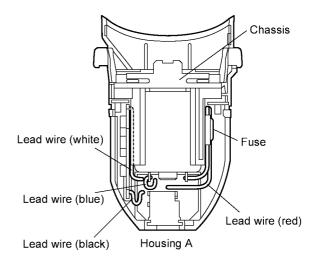
4. Close the housing A and B and tighten two screws after assembling housings with the bottom cover.
