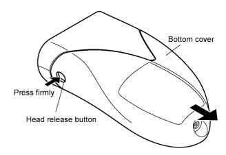
3. Separate the housing A and housing B with care to prevent breakage of hooks.
