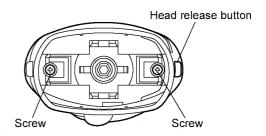
2. Take out the bottom cover with pushing a head release button.
