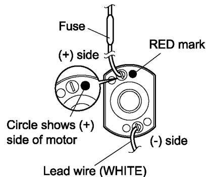
2. Put fuse onto the motor and fixed it with the motor cushion.
