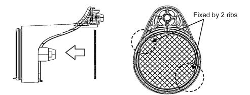
5. Install a MOTOR HEATER BLOCK ASS'Y, an AIR INLET RING, a LED COVER into HOUSING B.
