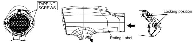
8. Set two TORX SCREWS (3.0\*12) at HOUSING A and fasten TAPPING SCREW (2.0\*4) at HOUSING C.
