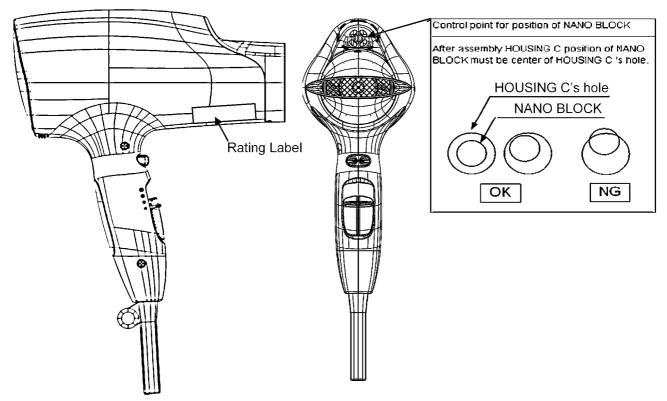
9. After assembly Mainbody and Nano effect must be Normal operate.
