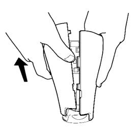
5. Remove MOTOR HEATER BLOCK ASS'Y and PLATE SPRING for FILTER FRAME BLOCK ASS'Y from AIR OUTLET RING, then remove AIR OUTLET RING as below.
