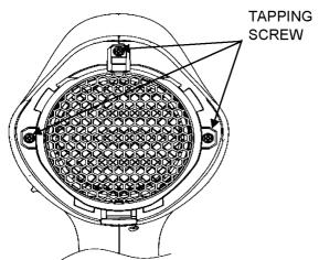
Remove TAPPING SCREW at HOUSING C by flat-blade screwdriver and two TORX SCREWS at HOUSING A by driver then remove HOUSING A.
