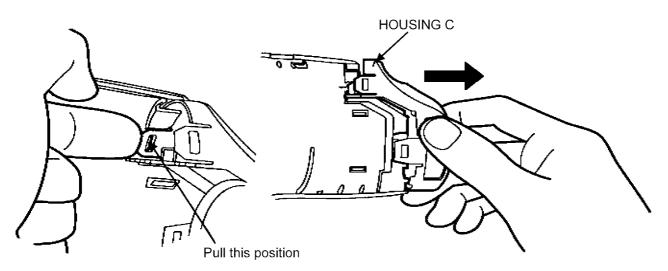
7. Remove NANO CIRCUIT BOARD ASS'Y from MOTOR HEATER BLOCK ASS'Y as below.
