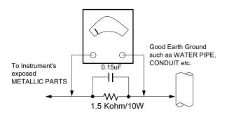
When 25A is impressed between Earth and 2nd Ground for 1 second, Resistance must be less than 0.1  $\Omega$  \*Base on Adjustment standard
