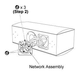
Step 3: Release the indicated nuts.Step 4: Remove the network assembly.
