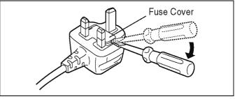
2. Replace the fuse and attach the Fuse cover.
