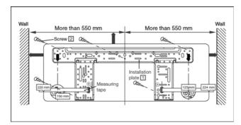
The centre of installation plate should be at more than 550 mm at right and left of the wall.
