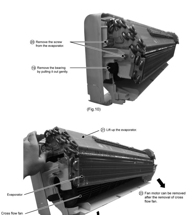
Remove the cross flow fan from the unit by pulling it to the left and downward.
