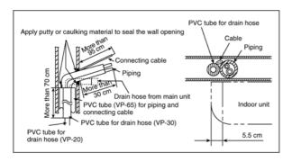
In case of left piping how to insert the connecting cable and drain hose.
