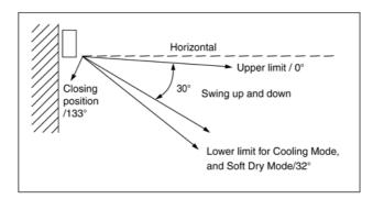
During Anti-Dew condensation prevention, the horizontal louver angle in Manual control are as below figure.
