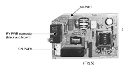
Detach the RY-PWR, AC-WHT and CN-PCFM connector from the electronic controller. Then, pull it slowly while pressing the fastener to the left.
