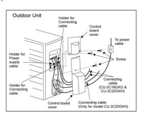
Note: Knife switch (Disconnecting means) should have minimum 3.5 mm contact gap. Secure the cable onto the control board with the holder (clamper).
