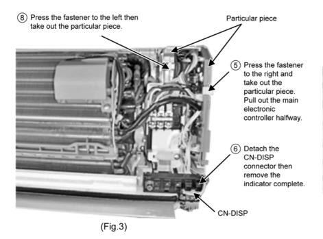
Detach 5 connectors as labeled from the electronic controller. Then pull out slowly while pressing the fastener to the right.
