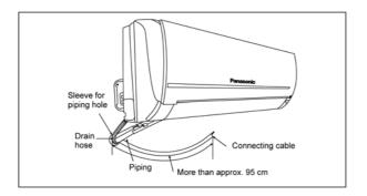
How to pull the piping and drain hose out, in case of the embedded piping.
