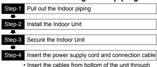
the control board hole until terminal board area.
