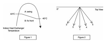
2 Manual horizontal airflow direction can be set using remote control; the angles of the vane are as stated below and the positions of the vane are as Figure 2 above.
