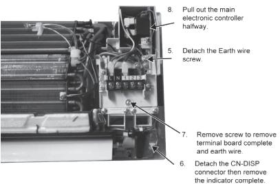
Detach connectors as labeled from the electronic controller. Then pull out main controller gently
