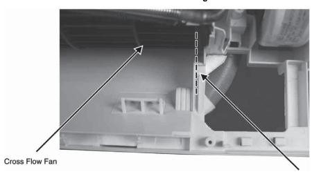
Reminder: To reinstall the cross flow fan, ensure cross flow fan is in line as shown in figure 10
