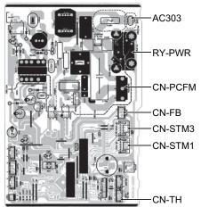
10 Detach AC303 (WHT) connector from PCB, then detach the RY-PWR (Black and Brown) from terminal board.
