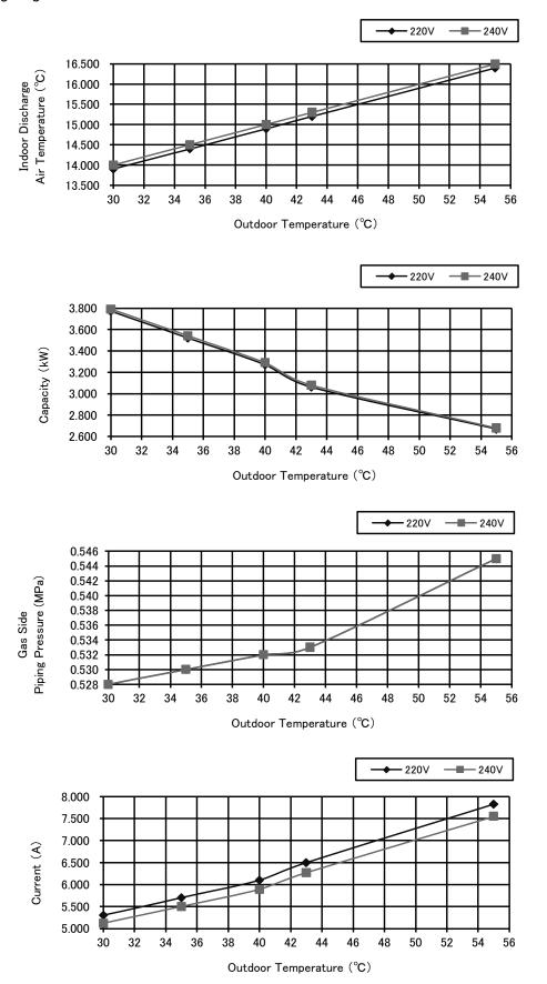
• Piping Length Characteristic Cooling
