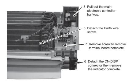
9 Detach connectors as labeled from the electronic controller. Then pull out main controller gently.
