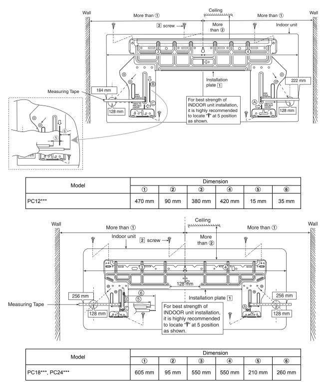
The center of installation plate should be at more than ① at right and left of the wall.
