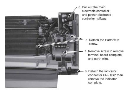
9 Detach 4 connectors as labeled from the electronic controller. Then pull out main controller gently.
