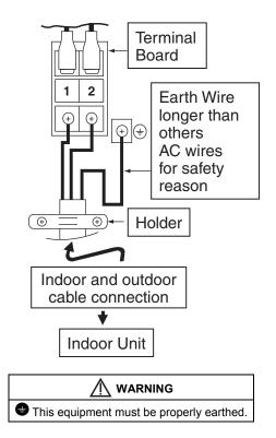
Earth wire shall be Yellow/Green (Y/G) in colour and longer than other AC wires for safety reason.
