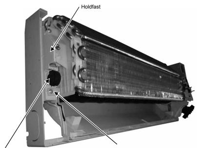
16 Remove the bearing by pulling it out gently. 15 Remove the 2 screw from the evaporator
