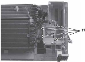
13 Remove 4 screws holding the control board then pull out the control board.
