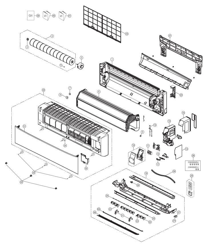
Note The above exploded view is for the purpose of parts disassembly and replacement. The non-numbered parts are not kept as standard service parts.
