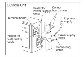
Note: Knife switch (Disconnecting means) should have minimum 3.5 mm contact gap.
