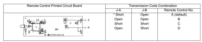
• Under various setting mode, after select the transmission code combination of remote control, press any button of remote control to transmit a signal to indoor unit. The transmission code will be stored in EEPROM.
