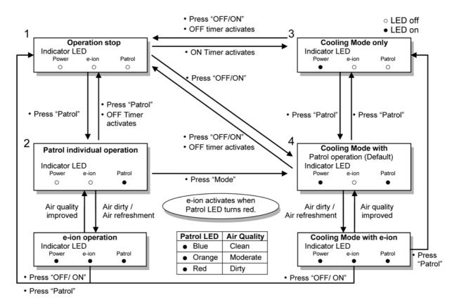
• To monitor air dirtiness level by using Patrol sensor and to maintain air freshness by activates e-ion operation.
