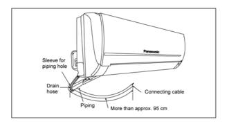
How to pull the piping and drain hose out, in case of the embedded piping.
