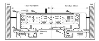
The centre of installation plate should be at more than 450 mm at right and left of the wall.
