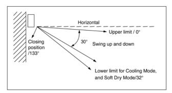
During Anti-Dew condensation prevention, the horizontal louver angle in Manual control are as below figure.
