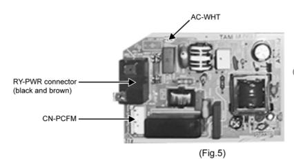
Detach the RY-PWR, AC-WHT and CN-PCFM connector from the electronic controller. Then, pull it slowly while pressing the fastener to the left.
