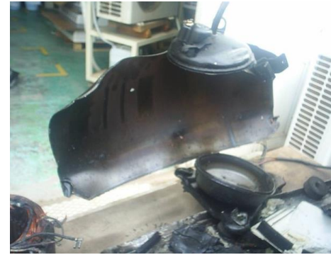
The ignition point start from the compressor
