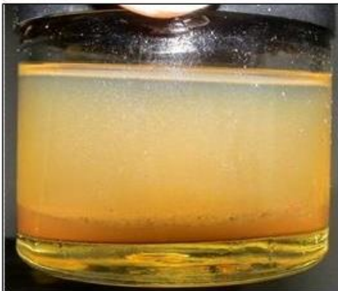
Comp. oil with rusty water
