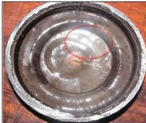
Lower shell oil with water
